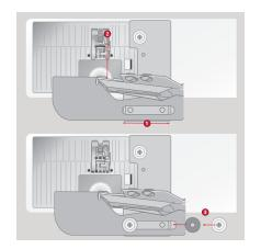
The Double Fold 1/2" (12mm) binder will turn a light weight woven fabric strip into a binding and attach it to the project edges all in one step when fitted with 412964206 or 412964207 stitch plate.
